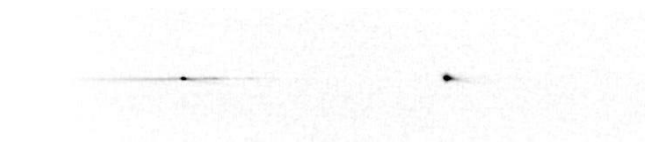
Figure 10 – Spectrum recorded at Gnosca. Meteor moving to the left, first order at other side of zero order compared to MAI_2, therefore the meteor train pointing in the other direction with respect to the spectrum. 50 fields added.
