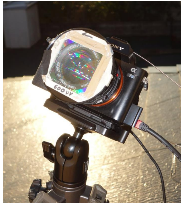
Figure 8, Sony alpha7s equipped with grating 600 grooves/mm software. In the future it is planned to simplify the calibration and to streamline the processing pipeline. This may help in popularizing meteor spectroscopy in the community. At present additional stations of the FMA plan the installation of meteor spectroscopy cameras in Switzerland. Since two years the FMA operates a network of video, fireball detection, radar and seismic stations, which in combination allow a better characterisation of meteors.
